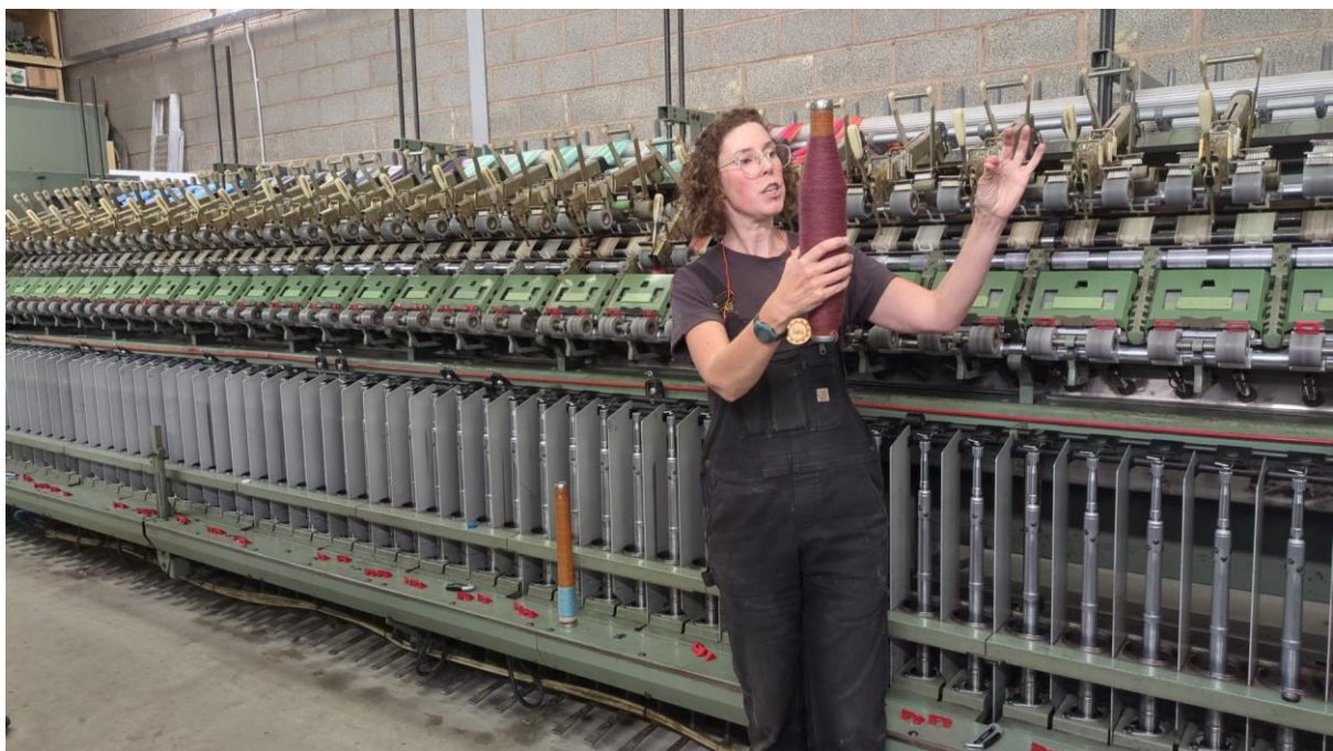
Kevin – The Draft Spinner with 96 spinning heads. Takes the Tops down to a single ply in one go.
