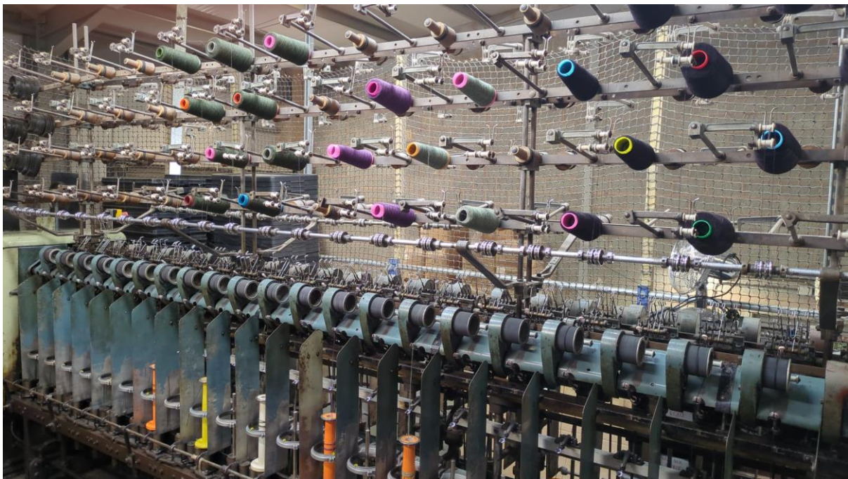
Mr Boyd - Plyer/Folder – Takes the single yarn and makes plyed yarn
